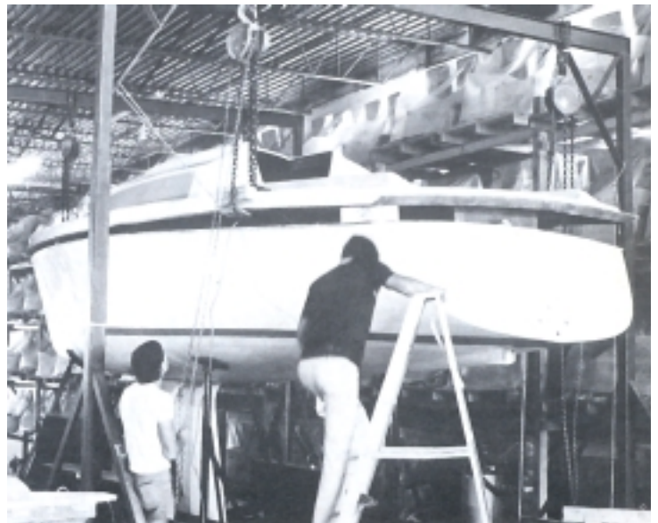
The prototype gets its trail cabin top at BYRD, summer 1982. (In the background are railway seats using the closed mould process.)
