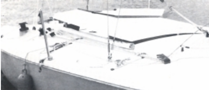
Prototype with large section of flush deck starting to be raised.
